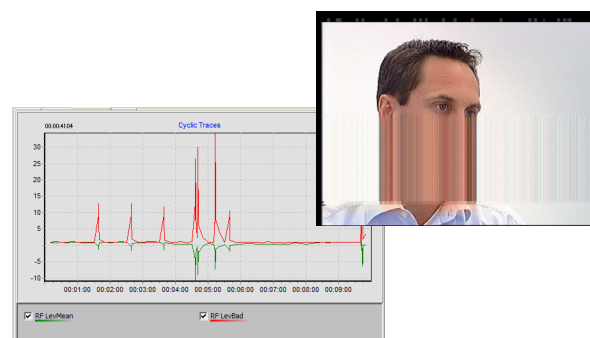
RF Traces plotted during ingest, indicating problematic transfer (e.g. due to damaged tape or smeared reading head of VTR).
