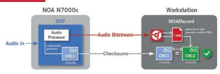
N7000c. BitProof works continuously in realtime during the active recording - with no additional operational overhead or intervention by an operator. Should an error occur, it will be detected and reported reliably, enabling the operator to react immediately. A domain of trust is established, starting from the A/D converter covering the complete transfer chain towards the recorded archive facsimile.
